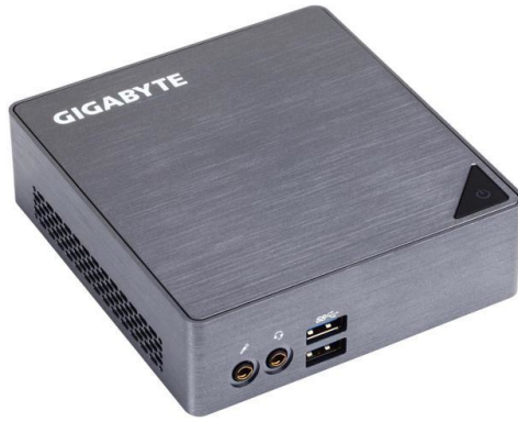
Figure 2.10: Gigabyte Brix i7-8550 onboard computer used to process mapping, estimation, and navigation algorithms.
