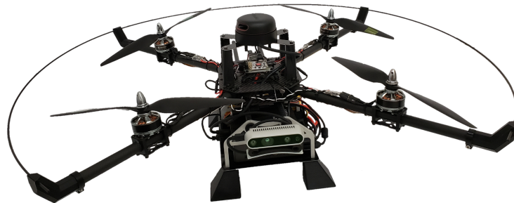
Figure 2.4: Customized Tarot LJI 500-X4 Quadrotor airframe built with sensors attached.
